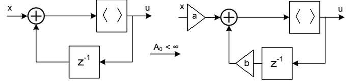
Fig. 6. Block model of the modulo integrator for finite DC gain.
