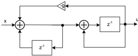
Fig. 12. Resonator based on the lossless discrete integrator (LDI)
