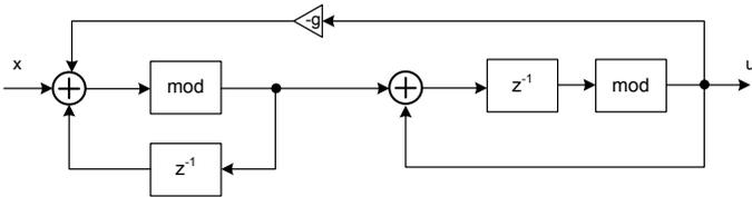
Fig. 13. The modulo resonator
