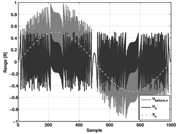
Fig. 3. States of the modulo integrator for a sinusoidal input  $x_n$ . The output before modulo is  $u_{before,n}$  and the output after is  $u_n$ .
