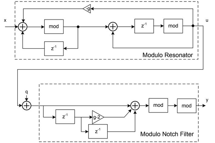
Fig. 14. The open-loop sigma-delta modulator with NTF zeros at non-zero frequency
