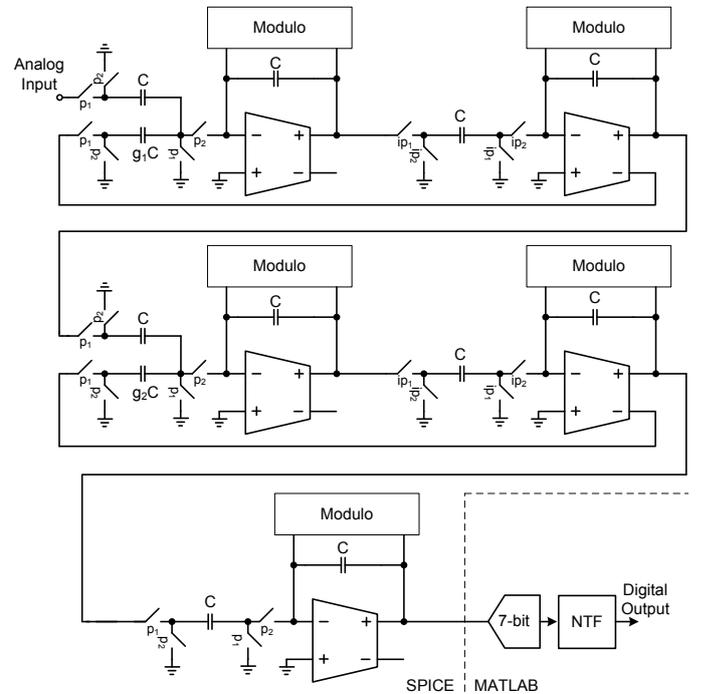
Fig. 20. Fifth order OLSDM SPICE model. Quantization and NTF are implemented in MATLAB
