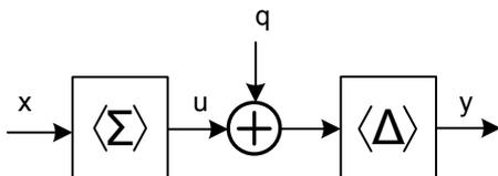
Fig. 1. First order low-pass open-loop sigma-delta modulator
