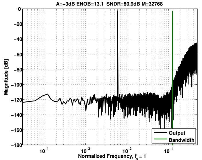
Fig. 19. Magnitude of a  $2^{15}$  point FFT of the modulator output. Input signal amplitude  $-3dBFS$ , input frequency  $f_i = 0.006$  and sampling frequency  $f_s = 1$ . With an  $OSR = 4$  the SNDR=80.9-dB
