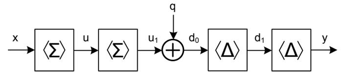
Fig. 2. Second order low-pass open-loop sigma-delta modulator
