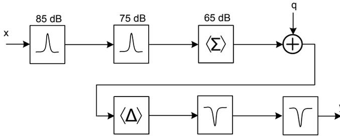
Fig. 18. Fifth-order open-loop sigma-delta modulator. The DC gain of opamps are shown above the stages.
