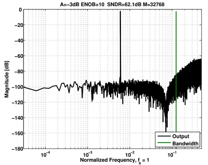
Fig. 15. Modulator response. Magnitude of a  $2^{15}$  point FFT. Input signal amplitude is -3dBFS, input signal frequency is at  $f_i = 0.006$  with a normalized sampling frequency,  $f_s = 1$ . The SNDR with  $OSR = 4$  is 62.1-dB
