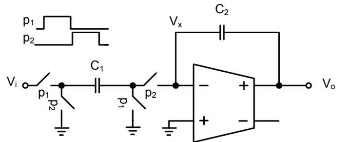
Fig. 4. Parasitic insensitive switched-capacitor integrator
