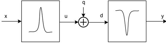
Fig. 11. Ideal open-loop implementation of NTF zeros at non-zero frequency
