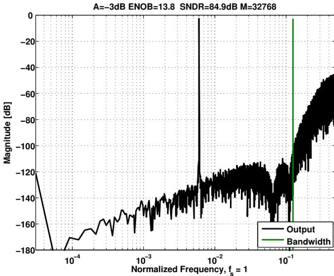
Fig. 17. Modulator output. Magnitude of a  $2^{15}$  point FFT of the modulator output. Input signal amplitude  $-3dBFS$ . Input frequency  $f_i = 0.006$  and sampling frequency  $f_s = 1$ . With an  $OSR = 4$  the SNDR is 84.9-dB
