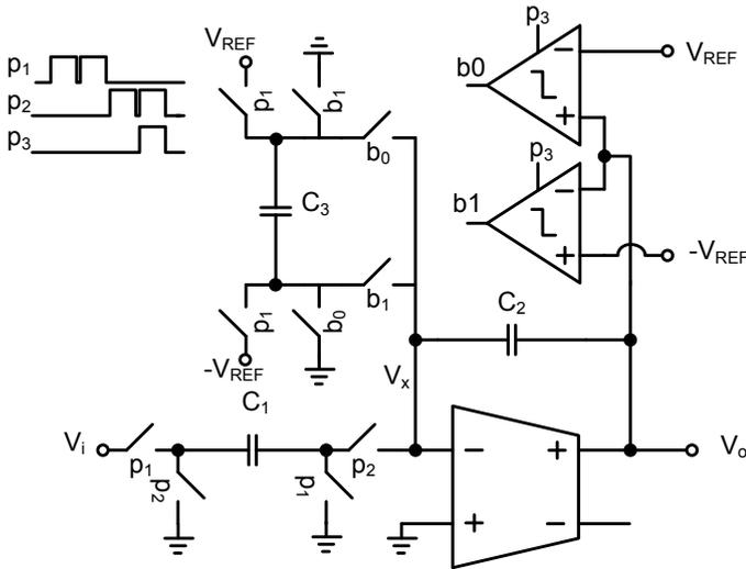
Fig. 5. Switched-capacitor modulo integrator
