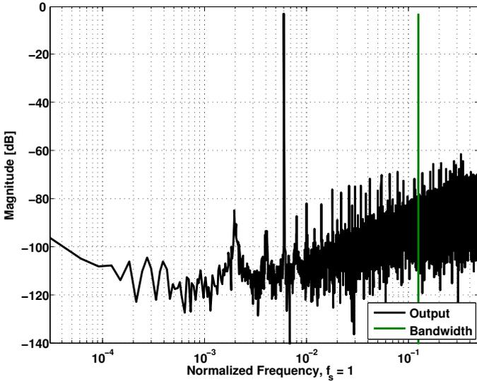
Fig. 7. SIMULINK model, SNDR = 52.20-dB
