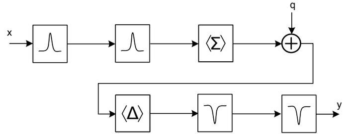
Fig. 16. Fifth-order open-loop sigma-delta modulator
