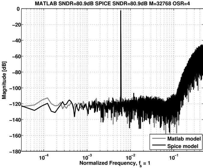
Fig. 21. Comparison of SPICE model and MATLAB model. Input signal amplitude  $-3\text{dBFS}$ , input frequency  $f_i = 0.006$  and sampling frequency  $f_s = 1$ . With an  $OSR = 4$  the SNDR is 80.9-dB for the MATLAB model and 80.9-dB for the SPICE model.
