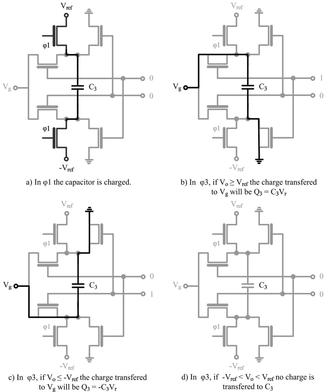
Fig. 12. The states of the modulo circuit in Figure 10
