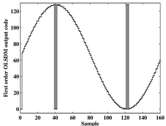
Fig. 6. The output of the first order OLSDM in the presence of *false modulo* errors
