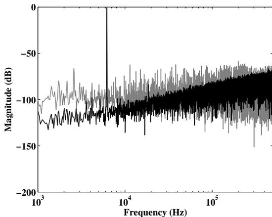
Fig. 15. FFT of output from first order OLSDM simulation in SPICE.
