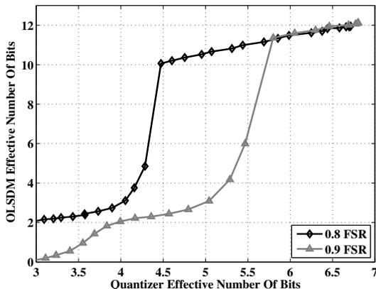
Fig. 7. Linearity of second order OLSDM as a function of quantizer linearity
