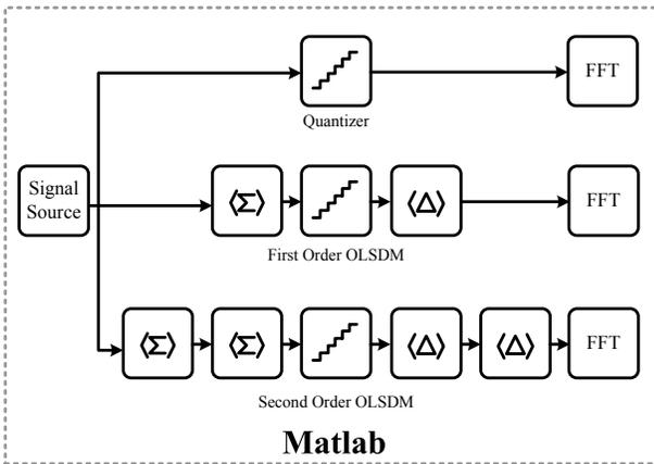
Fig. 3. Overview of behavioral level simulation system
