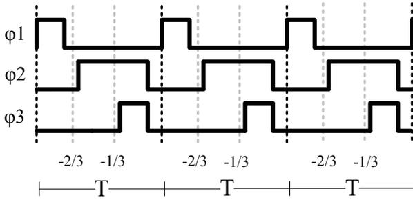
Fig. 11. Timing diagram for the modulo integrator
