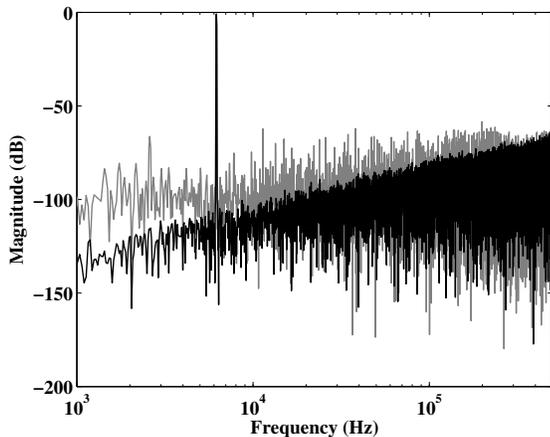
Fig. 4.  $2^{15}$  point FFT of the first order OLSDM output
