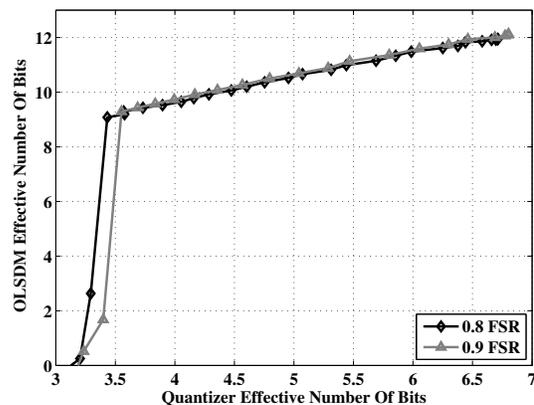
Fig. 8. Linearity of second order OLSDM as a function of quantizer linearity with error correction enabled
