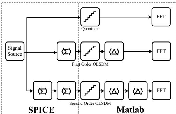
Fig. 13. Overview of circuit simulation with macro models
