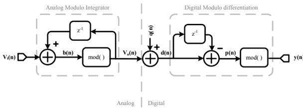
Fig. 2. Piecewise linear model of the OLSDM
