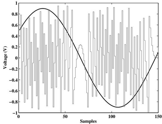
Fig. 14. Input vs output for the modulo integrator. Input is a sine with an amplitude of 0.9 V
