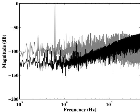
Fig. 16. FFT of output from second order OLSDM simulation in SPICE.
