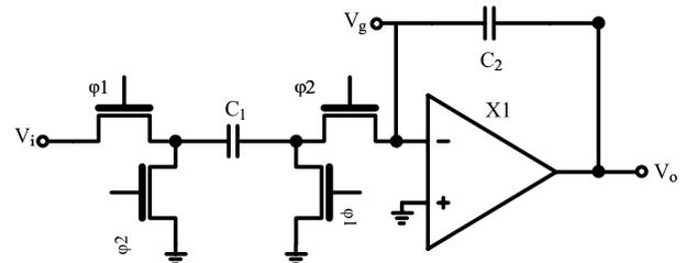
Fig. 9. Conventional switched capacitor integrator
