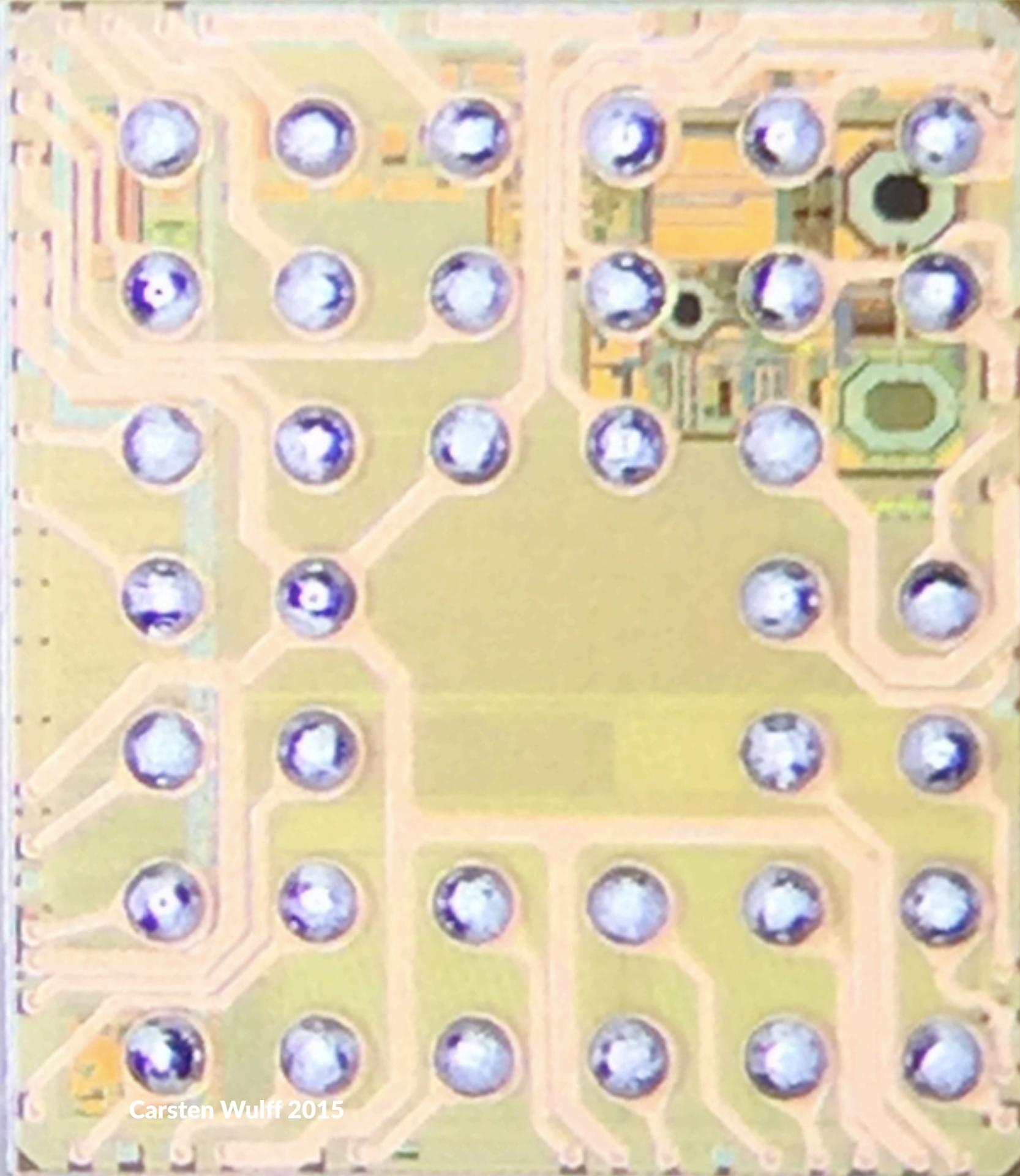
*analog/RF*: oscillators, bandgaps, noise generators, temperature sensor, linear voltage regulators, switch-mode voltage regulators, pad drivers, ADC, comparator, NFC, 2.4GHz radio
