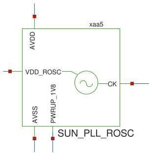
1) SUN\_PLL\_SKY130NM/sim/ROSC/: I simulate the ring oscillator in ngspice with a transient simulation and get the oscillator frequency as a function of voltage.
