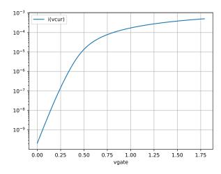
$$I = I_{D0} \frac{W}{L} e^{(V_{GS} - V_{th})/nU_T}, U_T = \frac{kT}{q}$$
