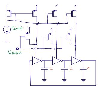
We can calculate the  $K_{vco}$  of the oscillator as shown below. The inverters mostly act as switches, and when the PMOS is on, then the rise time is controlled by the PMOS current mirror, the additional  $V_{control}$  and the capacitor. For the calculation below we assume that the pull-down of the capacitor by the NMOS does not affect the frequency much.
