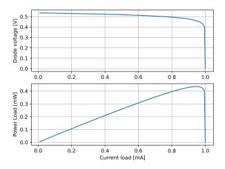
Most photovoltaic energy harvesting circuits will include a maximum power point tracker as the optimum changes with light conditions.
