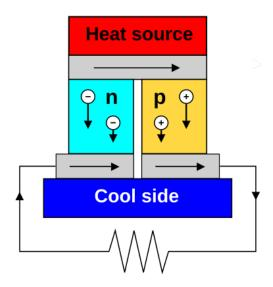
The process can be run in reverse. In the picture below we force a current through the material, we heat one end, and cool the other. Maybe you've heard of Peltier elements.
