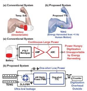
Below is some more details on the operation of the harvesting circuit, and the temperature sensor. Notice how the temperature sensor part of the circuit (PTAT bandgap, capacitor and comparator) produce a pulse width modulated signal that depends on temperature.
