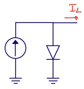
As the load current is increased, the voltage VD will drop. As the photo current is increased, the voltage VD will increase. As such, there is an optimum current load where there is a balance between the photocurrent, the voltage VD and the load current.
