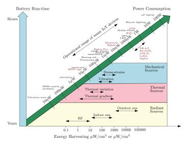
For wireless standards, there are some that can be run on energy harvesting. Below is an overview from [1]. Many of us will have a NFC card in our pocket for payment, or entry to buildings. NFC card has a integrated circuit that is powered from the electromagnetic field from the NFC reader.
