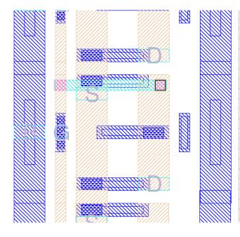
5) Drain of M2: Use the wire tool to draw connections for the drains.
