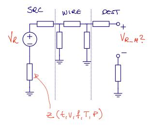
Most of the time, in order not to think about the ground impedance, we choose to route a known quantity as a current instead of a voltage. That means, however, we must convert from a voltage to a current, but we can do that with a resistor (you'll see later), and as long as the resistor is the same on the other side of the IC, then we'll know what the voltage is.
