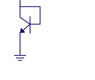
A diode connected bipolar transistor, or indeed a PN diode, assuming a fixed current, will have a voltage across that is temperature dependent
