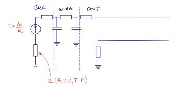
Resistors have finite matching across die, let's say 2 % 3-sigma variation. As a result, if we need a accurate voltage reference, then we must distribute voltage.
