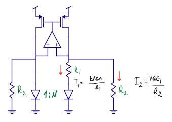
It does, however, change the current in the PMOS. Provided we scale  $R_2$  correctly, then the PTAT  $I_1$  can be compensated by the CTAT  $I_2$ , and we have a current that is independent of temperature.
