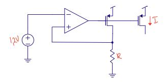
$$I_{D1} = \frac{1}{2}\mu_n C_{ox} \frac{W_1}{L_1} V_{eff1}^2$$
