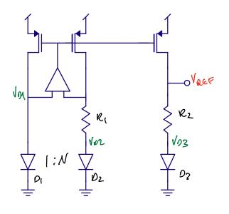
Another method would be to stack the  $R_2$  on top of  $R_1$  as shown below.
