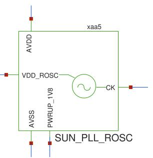
1) SUN\_PLL\_SKY130NM/sim/ROSC/: I simulate the ring oscillator in ngspice with a transient simulation and get the oscillator frequency as a function of voltage.
